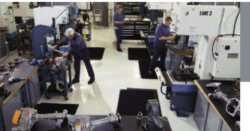
To support customer vehicle validation and testing, Dana builds thousands of axle and propshaft prototypes each year.
